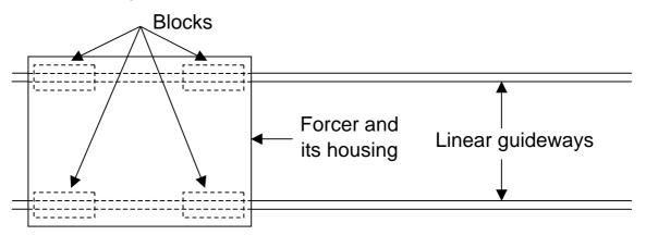
Figure 1. Installation of the forcer its housing
