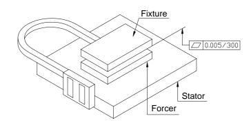
b. The foundation for the stator, its surface flatness must be less than 5µm/300mm, otherwise will cause stator to be bent also.
