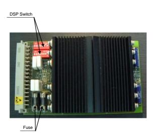
• The numbered PU2, PCB, the DIP switches have been set as followers: There are two DIP switches placed one is up and the other is down in parallel on each PU2 board.
