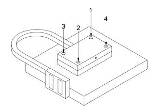
d. In the vicinity of the forcer avoid placing any strong magnetic material to effect the normal operation of the forcer.
