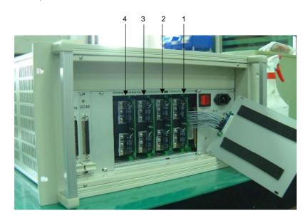
DIP switches and fuses on the PCB: The specification of the fuse is T6.3A/AC250V time lag type.
